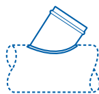
Shop/Field Installed Lateral Tap
