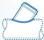
Shop/Field Installed Lateral Tap
